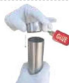
Use glue on top edge on end plug then insert in pipe & rotate once or twice clock and anti-clock wise.
